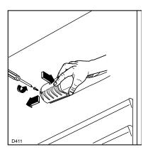
Unscrew the light cover and then pull it outward toward the middle of the cabinet. Unscrew the bulb and replace it with a new 15 watt bulb (available from your nearest Service Force Centre).
